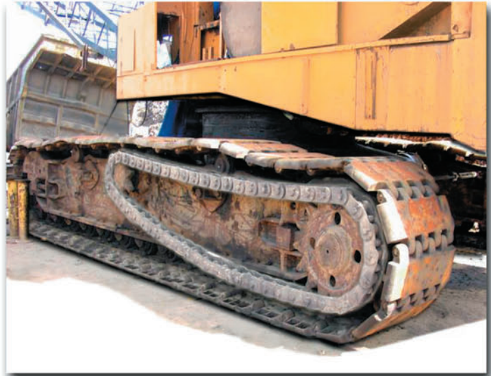
Engineering Class Drive Chain powers the crawler track of a crane. Note: For heavy duty, offset side bar style, engineering class drive chains, the correct running direction is to have the narrow end point toward the small sprocket on the "tight" (i.e. tension) side.
